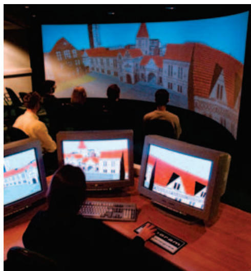
Figure 2: A large-scale, front projected, semi-immersive virtual environment.
