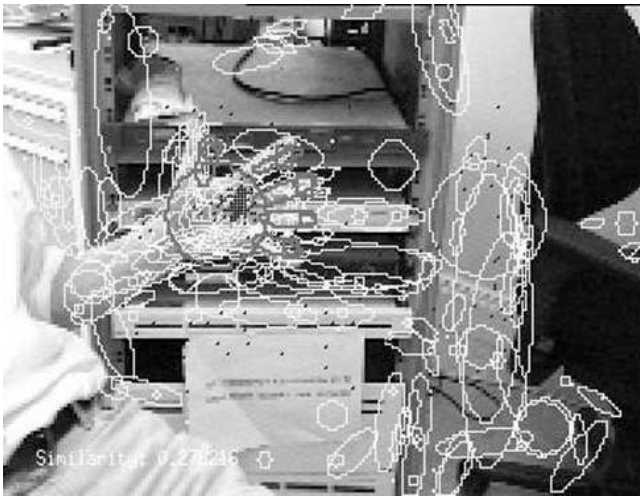
Fig. 1 Detected multi-scale features and the recognized hand pose superimposed in an image of a complex scene.
