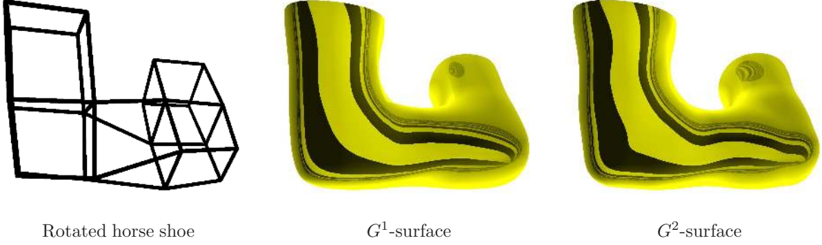
Fig. 5. Example of a quadrilateral mesh and the resulting G^1 and G^2 -surfaces with reflection lines.
