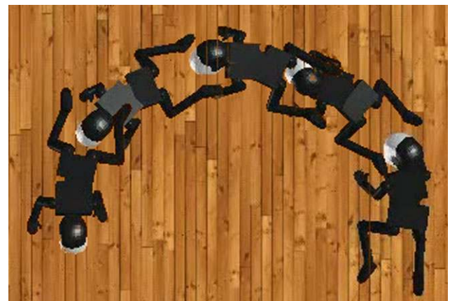
Fig. 23 The iCub turning. Superimposed snapshots of the robot turning with a torso angle of 0.5 radians. Movie available as Online Resource, Movie 6
