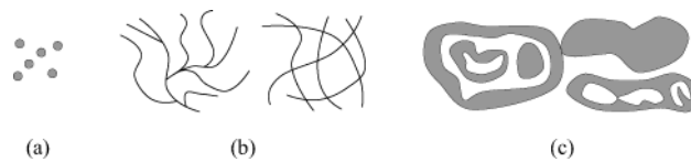
Fig. 3. Examples of a complex point object (a), a complex line object (b), and a complex region object (c).
