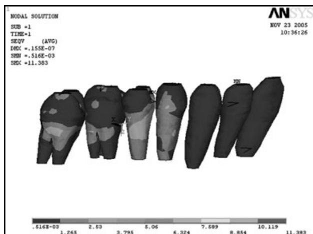
Fig. 8. Stress on the remaining teeth (model 2).
