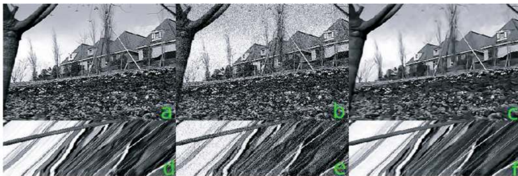
Fig. 5. Sequence “Flower garden.” (a) One image of the original sequence. (b) The same image of the noisy sequence with an additive Gaussian white noise of standard deviation \tau = 30 (PSNR = 18.58 dB). (c) The corresponding image of the denoised sequence, PSNR=23.59 dB. (d), (e), and (f) represent corresponding XT slices in the space-time domain. The camera motion induces lines in the XT slices.
