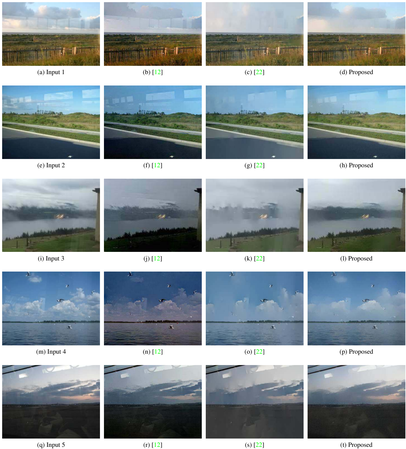
Figure 6. Comparison of reflection removal methods on real-world images taken from the Internet. As in the case of artificial images (Fig. 5), the method of Li and Brown [12] in the second column suffers from poor color reproduction, while the method of Wan et al. [22] in the third column over-smooths the image. Our method in fourth column gives superior color reproduction and reflection suppression results compared to both the state-of-the-art techniques. Best viewed on screen.
