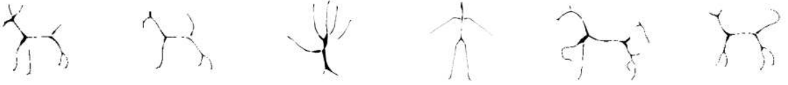
Fig. 10. Rough skeletons computed with \tilde{\Psi} . To obtain narrow skeletons we used a threshold, and repeated the computation of \tilde{\Psi} on the obtained region.
