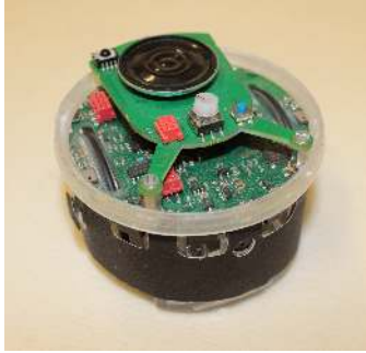
Figure 1: The e-puck robot fitted with a black ‘skirt’. The e-puck’s diameter and height are approximately 7.4 cm and 5.5 cm, respectively.
