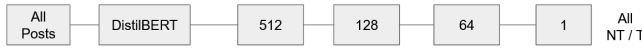
Figure 1: Architecture for Single Task, where all posts are passed through a neural network and get classified as toxic vs. non-toxic.
