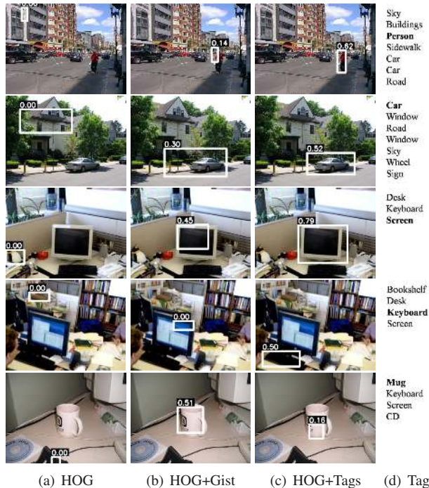
Figure 6. Example detections on LabelMe on five different target objects. Each image shows the best detection found; scores denote overlap ratio with ground truth. The raw appearance-only detector is confused by similar textures anywhere in the image (rows 1 and 2), whereas the detectors modulated according to the visual or tag-based context are more accurate. The Gist baseline usually gives good y estimates, while our method often provides a better scale estimate, particularly for indoor objects. When scene complexity (texture) is high throughout the image, Gist tends to be misled into predicting a too-small scale for the target object (row 4). Our approach can be misled on the scale prediction when the tags mention larger objects that are only partly visible (row 5).
