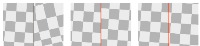
Figure 2: Behavior of various classes of parametrizations across cuts (red). Left: arbitrary transitions. Middle: so-called “seamless” parametrization with rigid transitions with rotational continuity across the cut. Right: quantized, integral parametrization.
