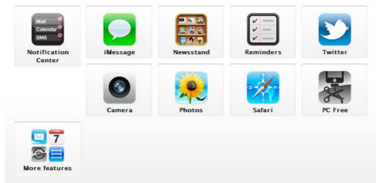
Figure 3.1.1. Surprises arise when indirect layout constraints do not entail the desired specifications. The oversized icon shifted the second row, rather than localizing the effect of its oversize.
