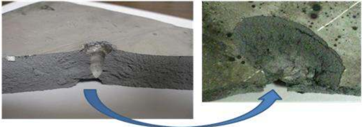
Figure 41. Photograph of the failed sample “A” after high strain impact.
