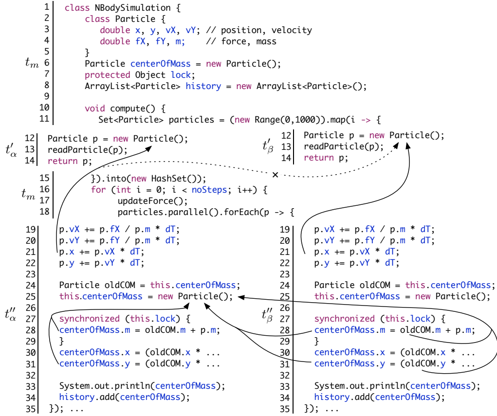
Figure 2: Visual representation of how our analysis sees a simple N-body simulation implementation. Each block of code is labeled with the abstract thread that executes it, e.g., t'_\alpha . The arrows show points-to relations from variables to allocation sites, e.g., variable p at line 21 in thread t'_\alpha may point to the abstract object instantiated on line 12 in thread t'_\alpha . Only relevant points-to relations are shown. The dashed crossed arrow represents an abstract points-to relation that would not appear in any real execution, so it is correctly missing in our model.
