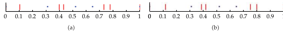
Figure 12: Parameter and knot distribution of (a) exponential and (b) proposed parameterization method.
