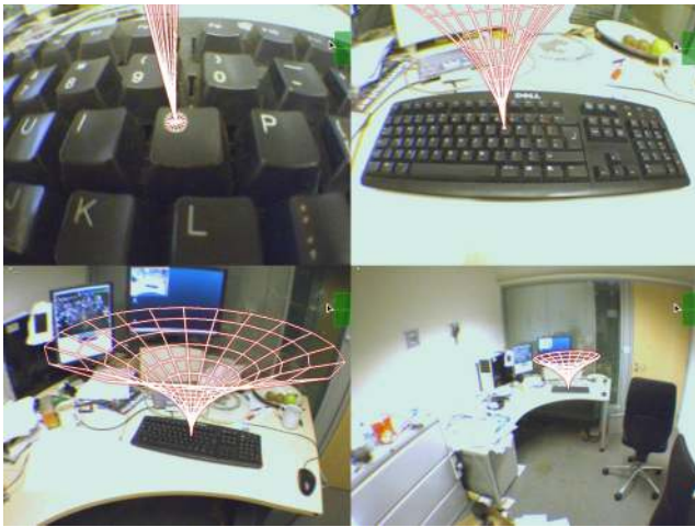
Figure 6: The system can easily track across multiple scales. Here, the map is initialised at the top-right scale; the user moves closer in and places a label, which is still accurately registered when viewed from far away.
