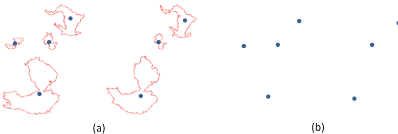
Fig. 1. (a) Objects are easy to match even with local deformations. (b) Points (centroids of lakes) are difficult to match.
