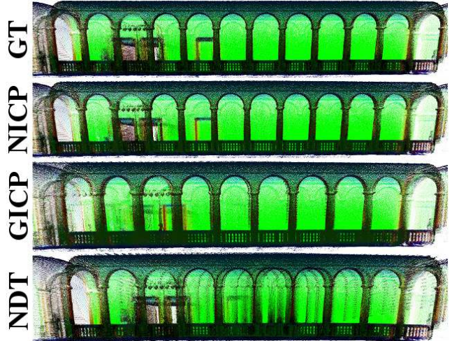
Fig. 1. Side views of the reconstruction of the ETH Hauptgebäude dataset. From top to bottom: ground-truth, NICP, GICP and NDT reconstruction. NICP was able to reconstruct consistently the scene while both NDT and GICP generated a shortened corridor ( count the arcs ).
