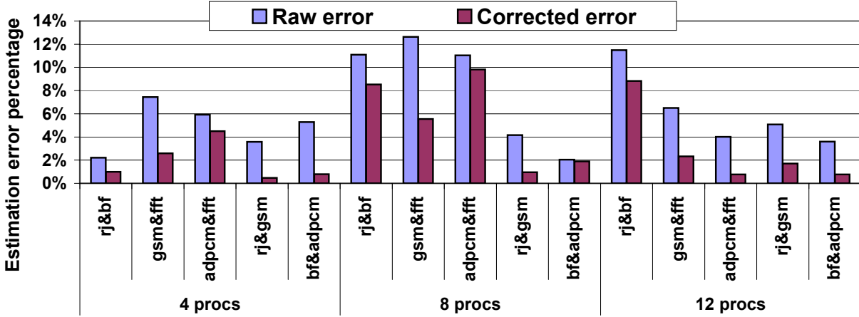
Figure 5: Estimated IPC error for 15 combinations. The number of processors varies from 4 to 12. The TWSS is set at 20%.
