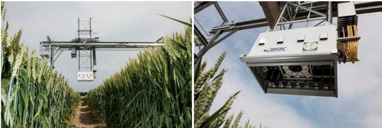
Fig. 2 Field Scanalyzer. (Left) The Field Scanalyzer phenotyping platform at Rothamsted Research showing (Right) the cameras within the camera bay directed down, perpendicular to the ground
