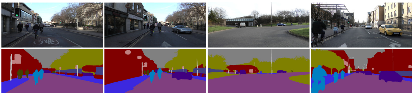
Figure 11. Output produced by (a) ContextNet, (b) FAST-SCNN, (c) FANet, (d) MCANet using CamVid validation image
