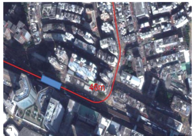
Figure 1. Horizontal curve design of monorail [13]
