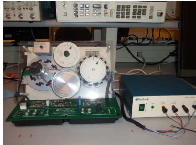
Figure 2. Servo mechanism plant with power supply
