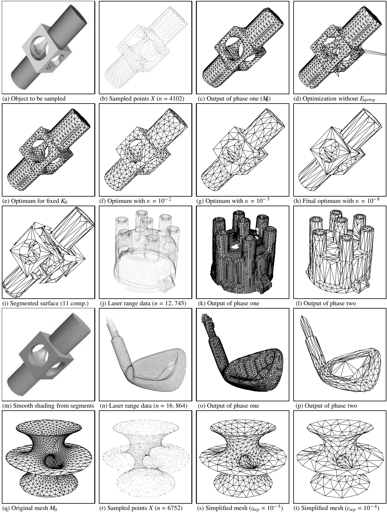
Figure 7: Examples of surface reconstruction and mesh simplification.
