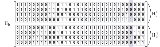
Fig. 4. Parity check matrix of an LDPC code optimized for super-code based decoding.
