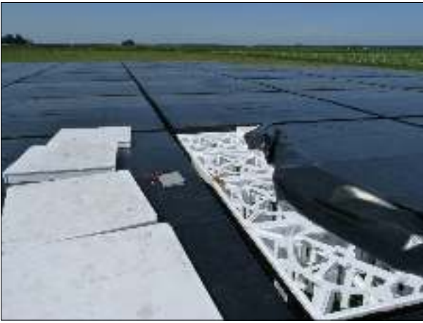
Fig. 7. Left: closeup image of a single LOFAR HBA tile. The protective covering has been partially removed to expose the actual dipole assembly. The circular dipole rotation mechanism is visible. Right: median averaged spectrum for all HBA tiles in station CS003. Various prominent RFI sources are clearly visible distributed across the band including the strong peak near 170 MHz corresponding to an emergency pager signal.
