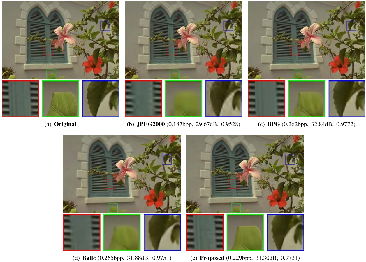
FIGURE 4. Visual comparison of the test methods on the Leaves image (bits per pixel, PSNR, MS-SSIM).
