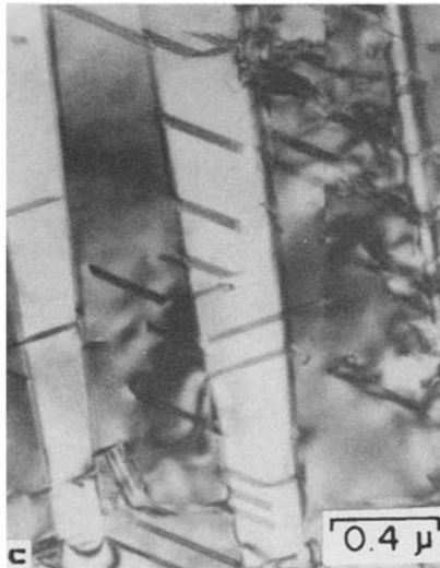
Figure 2. (a) Unit cell of \text{DO}_{22} structure, (b) [001] projection of perpendicular twins and (c) lenticular shaped twin lamellae of \text{Ni}_3\text{V} variants; \{110\} is the twin plane.
