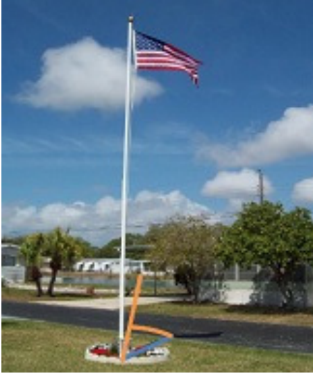
Fig. 4. offset angle is the angle between the shadow (blue) and the camera's optical axis (orange), measured in the ground plane.
