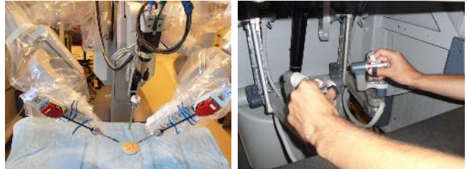
Fig. 1. Configuration of the da Vinci robot: patient side manipulators plus endoscopic camera (left) and master manipulators (right).
