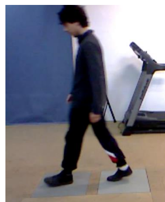
Figure 19: One of the subjects during the walking test on the force platforms in the UPC Biomechanics Laboratory
