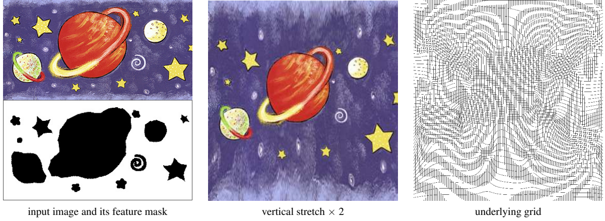
Figure 3: Feature-preserving stretching. The mapping preserves the shape of the features at the expense of the background.
