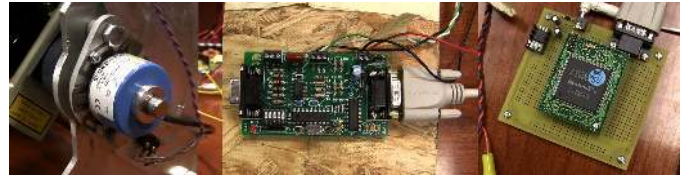
Fig. 5. This control system, consisting of a rotary encoder, pulse counter, and real-time polling software, was assembled as a platform for hardware-in-the-loop experimentation with interactive WCET analysis.
