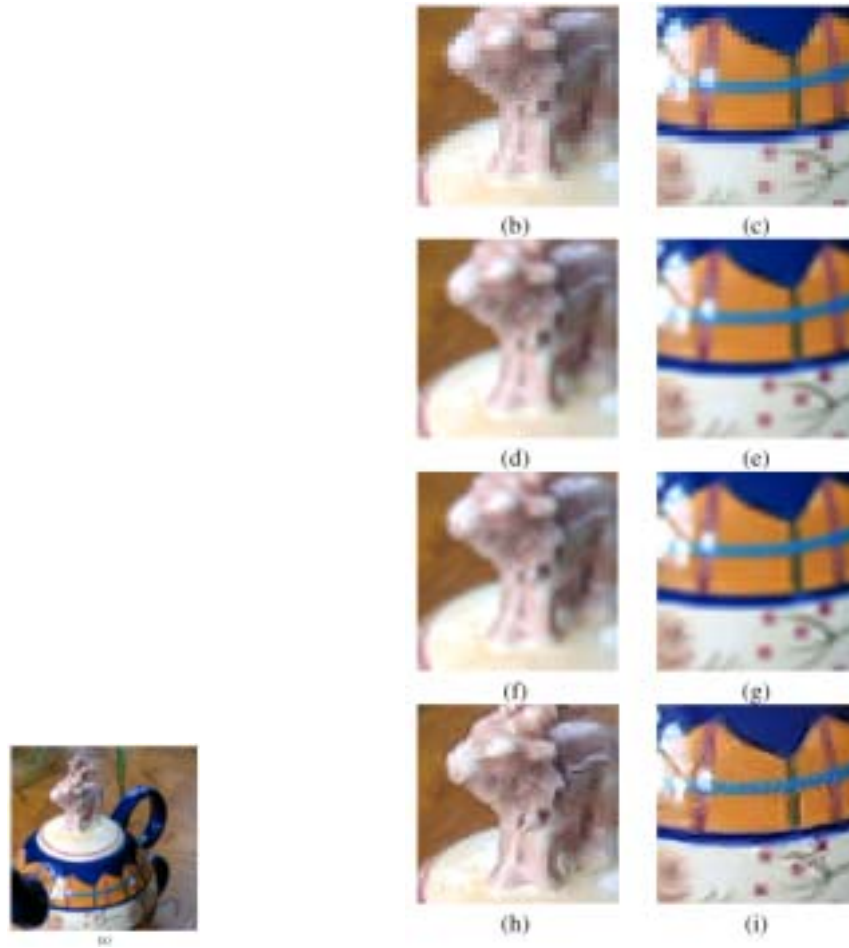
Figure 1: (a) An image (100x100) of a real-world teapot shows a richness of texture, but yields a blocky or blurred image when zoomed in by a factor of 8 in each dimension by (b, c) pixel replication or (d, e) cubic spline interpolation. (Images (b) through (i) were 32x32 pixel original sub-images, zoomed by 8 to 256x256 images). Sharpening the cubic spline interpolation may not help to increase the perceptual sharpness (f, g, using “sharpen more” in Adobe Photoshop). (h, i) show the results of our example-based super-resolution algorithm, maintaining edge and line sharpness, and plausible texture details.
