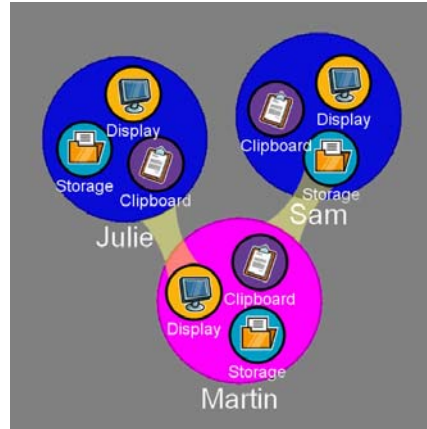
Figure 5: Join-the-dots graphical user interface (GUI) used to manually create compositions by sharing resources with a simple line drawing metaphor. This interface has been designed to work well with touch-screen or pen interfaces, and does not rely heavily on detailed manipulation or textual input.
