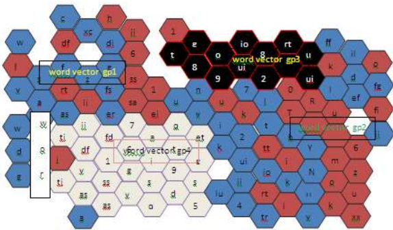
Fig 2: SOM for clustering closer words and to plot histogram with number of occurrences in the document. Note closer words are clustered into one word by SOM.
