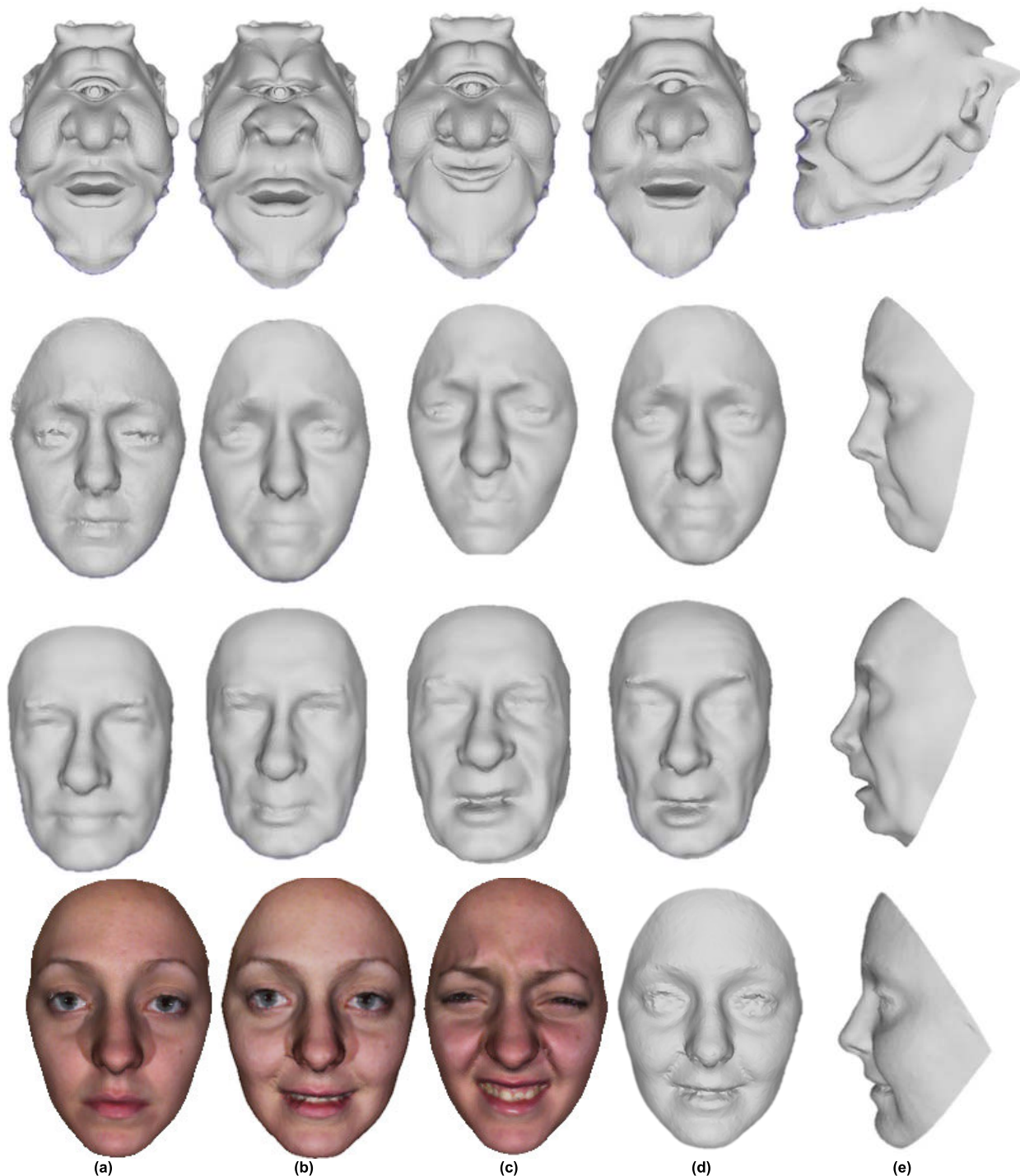
FIGURE 12. Results of face model editing algorithm (a) Source models; (b) Target models 1; (c) Target models 2; (d) Resulting Models; (e) Resulting models from a different perspective.
