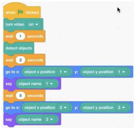
Fig. 8. Simple Program to Detect Object using the Pre-Trained Object Detection Model
