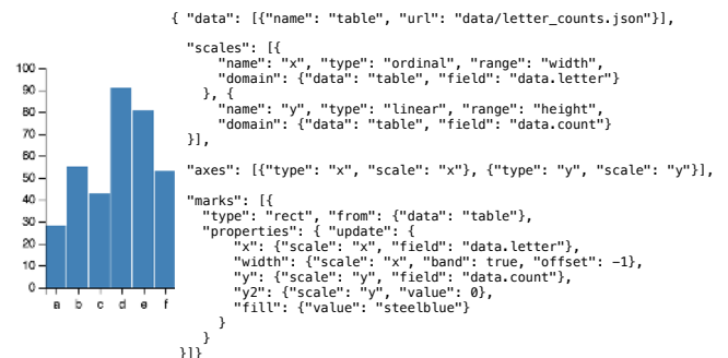
Figure 1. A JSON specification for a bar chart, demonstrating Vega’s [36] existing abstractions. Data is imported from a URL. Scales are defined to transform data values to visual values. Properties of graphical marks (in this case rectangles) are determined by scale mappings. Guides (here, axes) can be instantiated as well.
