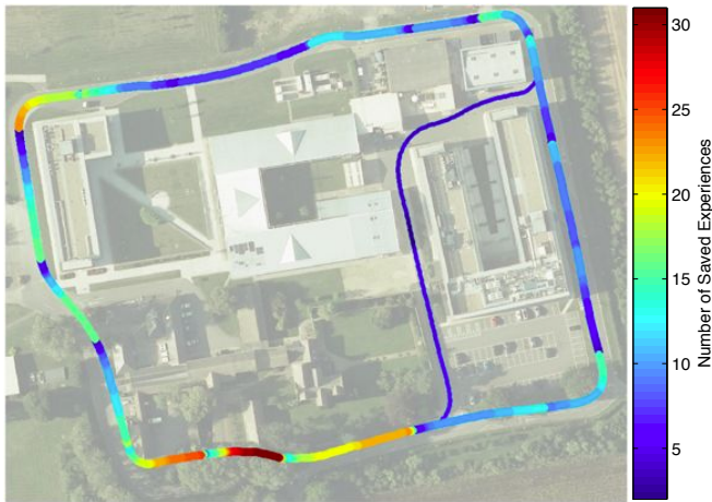
Fig. 3. An overhead of the Begbroke site, including the two loops driven over the three month period. The outer loop was driven 47 times (thicker line). The inner loop (thinner line) was driven 6 times. The colour of the plot at each point indicates how many experiences are stored there. This figure is reproduced from [1].
