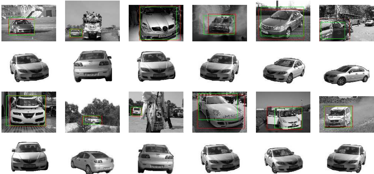
Figure 6. Pose estimation examples. The figure shows green bounding boxes around cars identified by our method. Ground truth bounding boxes are shown in red. In addition, below each image we show the car from the initial set whose view was found closest by our method.
