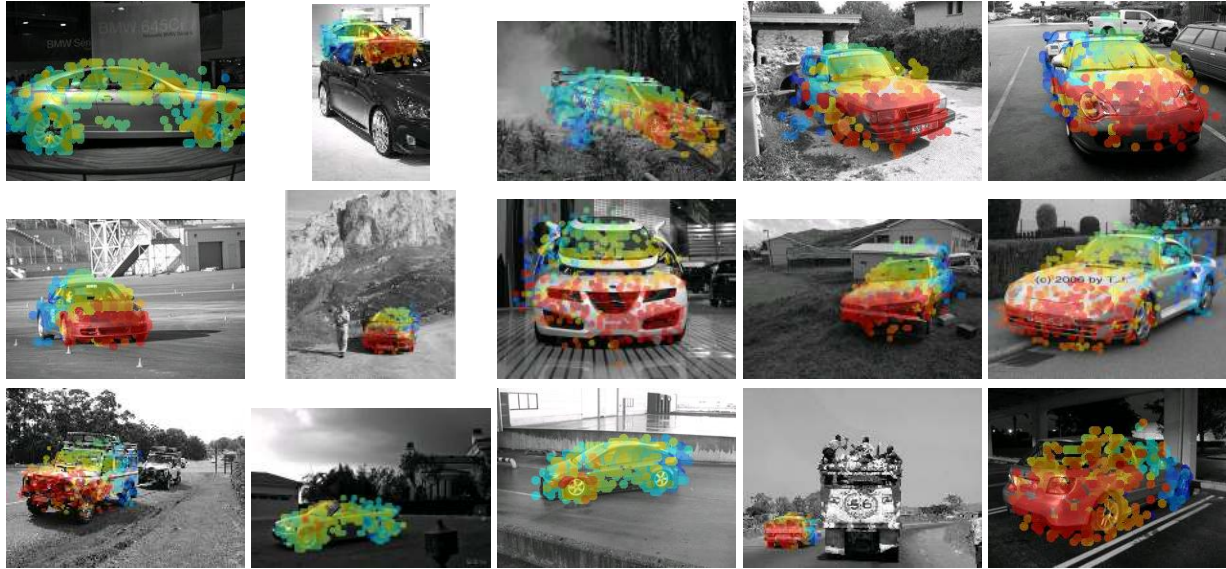
Figure 9. Depth values of features predicted by the model. Color values vary from red (closer to the camera) to blue (further from the camera).
