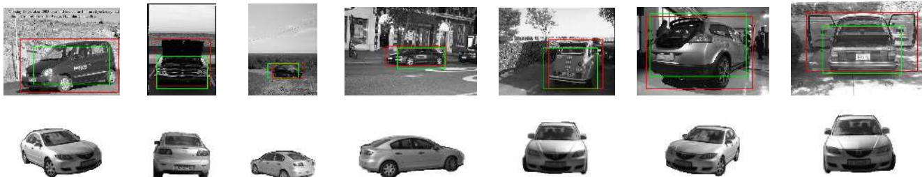
Figure 7. Pose estimation errors. The figure shows green bounding boxes around cars identified by our method. Ground truth bounding boxes are shown in red. Below each image we show the car from the initial set whose view was considered closest by our method.
