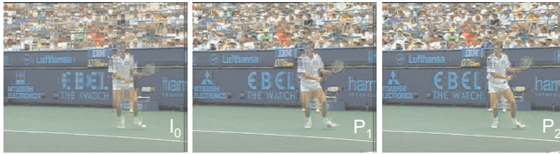
Figure 6.7: Gradual reduction of coding artifacts in time for interframe coding using a scalable DCT.
