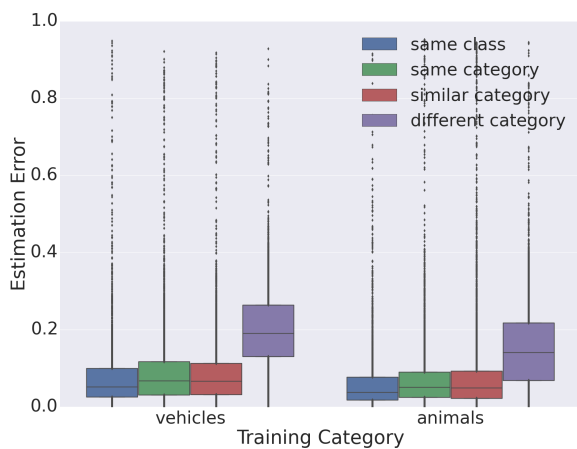
Fig. 10: Descriptive statistics of the quality estimation error when training on animals or vehicles and testing on (1) the same class, (2) the same category (here: different animals or vehicles), (3) a similar category (here: vehicles or animals) and (4) a different category (here: rectangular-shaped objects).
