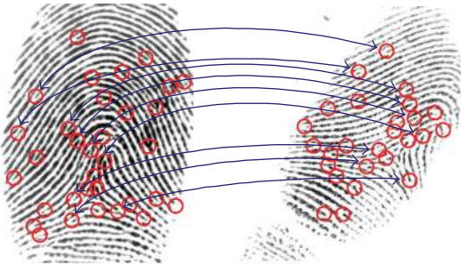
FIGURE 4: Illustration of biometric intraclass variability. Two different impressions of the same finger obtained on different days are shown with minutiae points marked on them. Due to translation, rotation, and distortion, the number and location of minutiae in the two images are different. The number of minutiae in the left and right images is 33 and 26, respectively. The number of common minutiae in the two images is 16 and few of these correspondences have been indicated in the figure.
