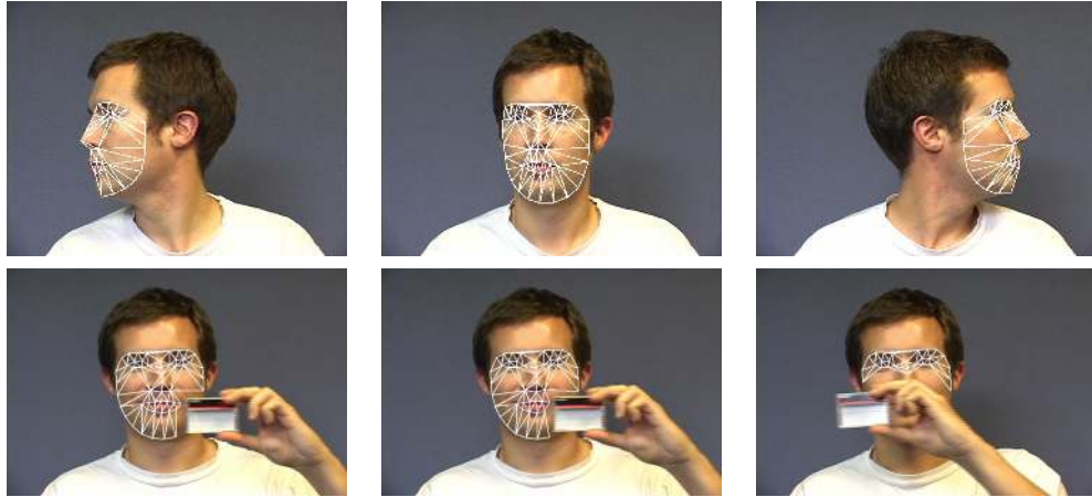
Figure 6: Training images with and without occlusion. We show 6 of the 120 hand-marked images used in the training of the AAM for the tracking task of Figure 7.
