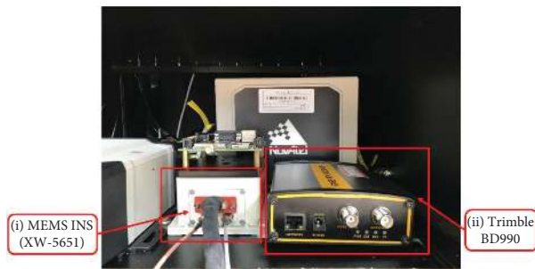
FIGURE 5: The MEMS INS and BDS receiver for verifying the proposed algorithm. (a) The MEMS INS XW-5651. (b) The GNSS receiver Trimble BD990.
