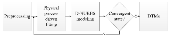
FIGURE 1. Framework of the physical process driven DTM generating method based on D-NURBS.
