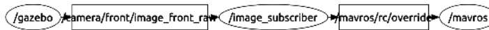
Fig. 7. Diagram generated by the program rqt_graph showing the relevant nodes and topics in the application
